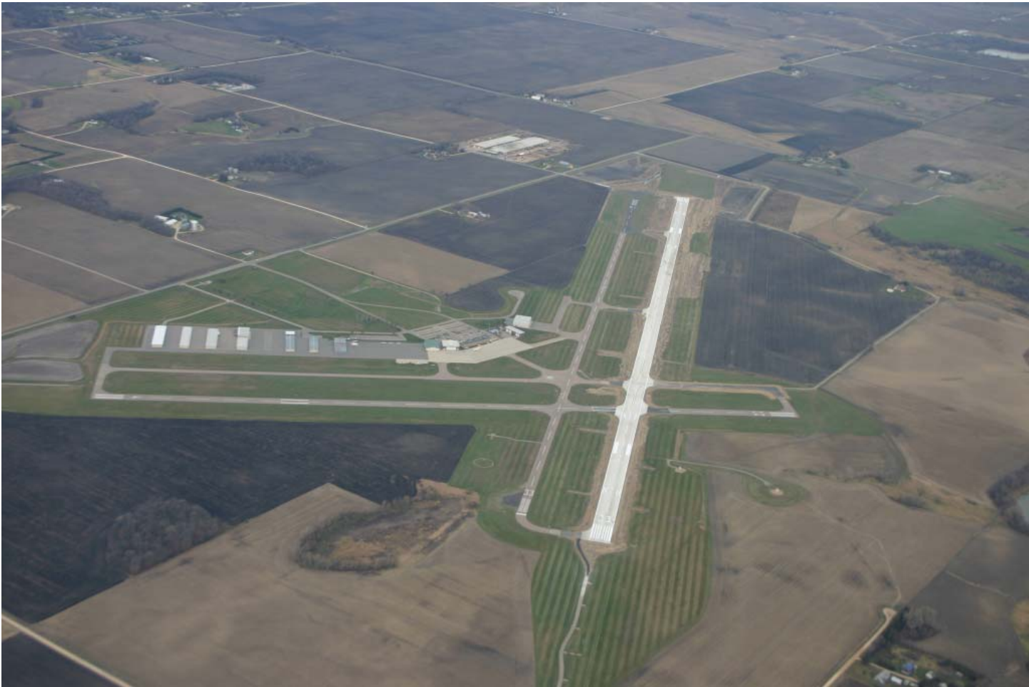
Mankato Regional Airport...Runway 15-33 is extended from 5,400 to 6,600 feet, which will now accommodate airplanes as large as a 757.
